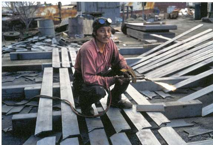
SHIPYARD WELDER CUTTING STEEL FOR HYUNDAI TRUCK CHASSIS, ENSENADA
